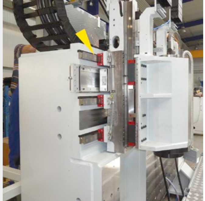
ACE clamping and safety elements maintain a rock-solid hold on the axes in special lathes and secure the predetermined positions both horizontally and vertically RASOMA Werkzeugmaschinen GmbH, 04720 Döbeln, Germany
