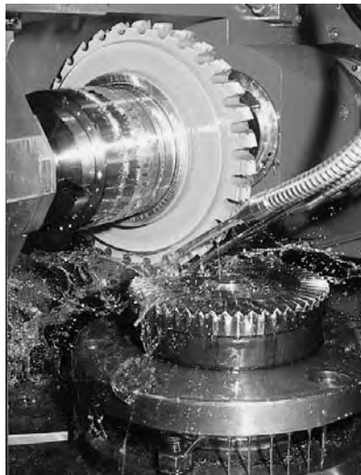
CNC Machining of a PowerTRUE™ right angle gear
