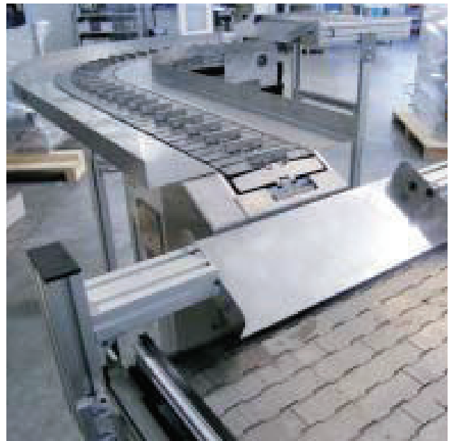
Flat top chain conveyors for transporting hot products
