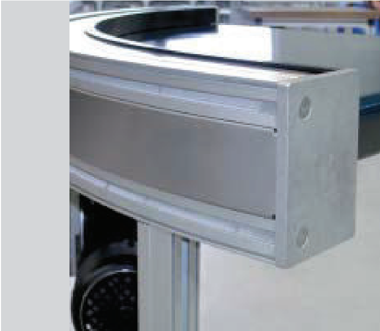
The flat, side end of the KGF-P 2040 ensures short transfer paths
