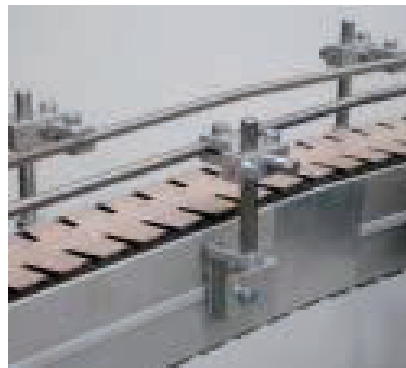
Short vertical bend for forming a storage area with several levels
