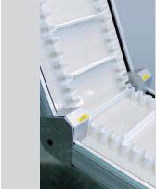
Inclined conveyor with FDA belt and sidewalls
