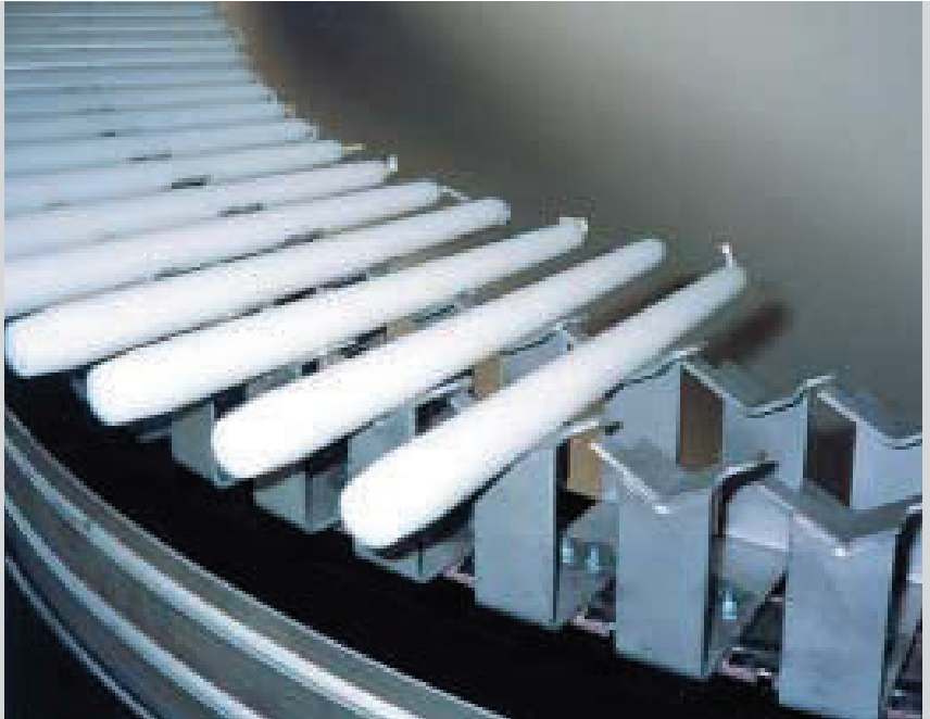
Multiflex Chain Conveyor with special fixtures for moving candles
