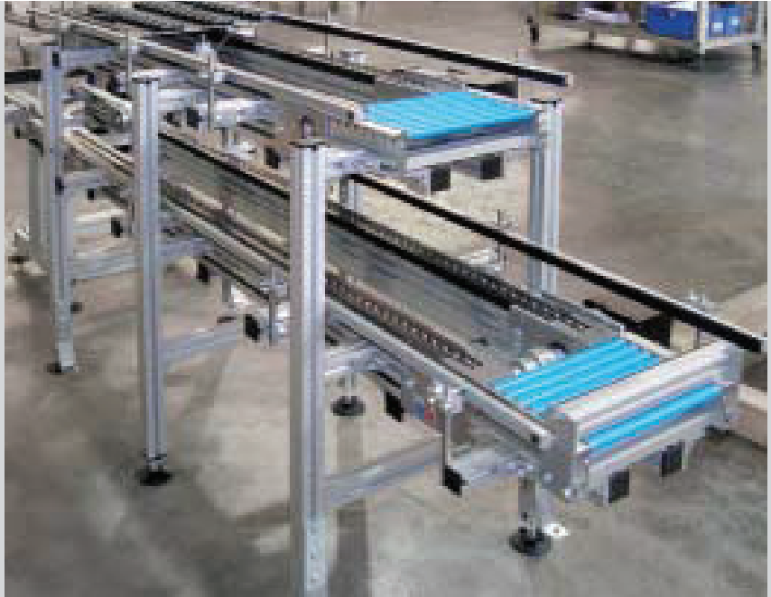
Accumulating roller chain conveyors with infeed and outfeed segments
