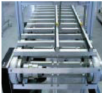
ZRF-P 2040.02 with customer-specific side rail for parallel conveying of two workpieces
