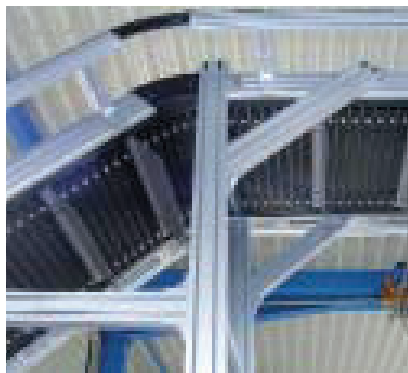
Solid support of the KFM-P 2040.86 for conveying heavy loads
