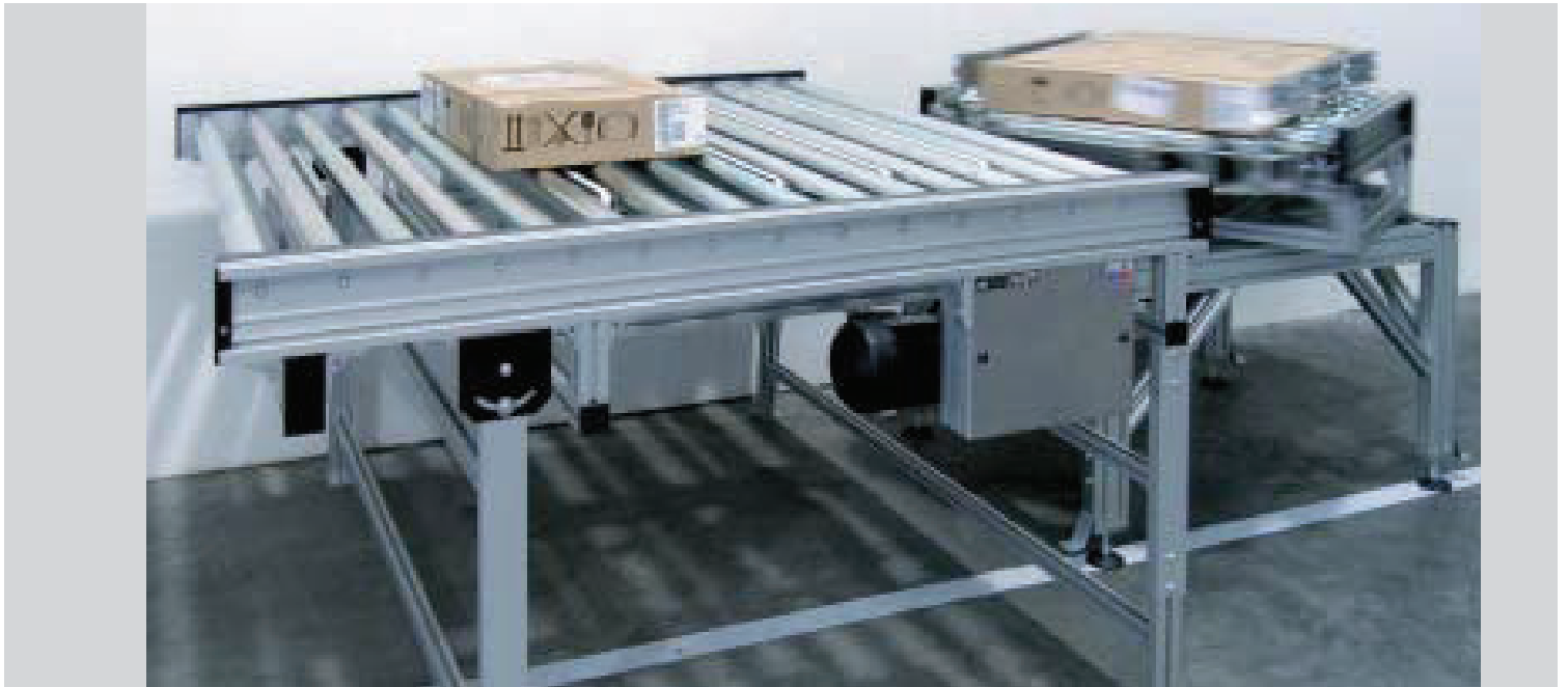
Combination of turn table and RBT-P 2255 with buffer table for order picking tasks and \varnothing 50 mm steel rollers. Driven via tangential chain drive
