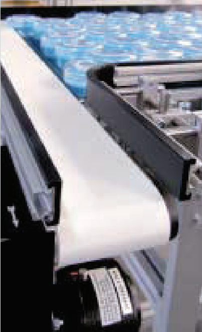
GUF-P 2000 as transverse conveyor and singulator following a cooling section
