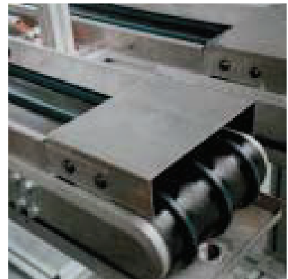
GUF-P 2041 with drip pan and longitudinal cleats
