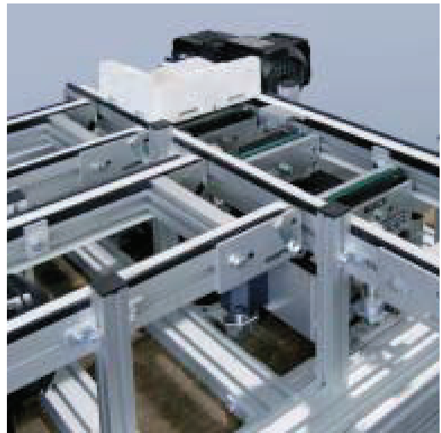
Dual-lane conveyor 2001 with integrated lift and transfer station
