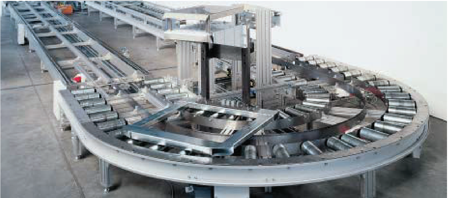
Special roller conveyor for transporting pallets integrated in a complete system
