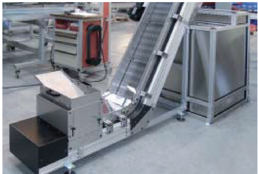
KFM-P 2040.86 for hot products with changeable size parts reservoir
