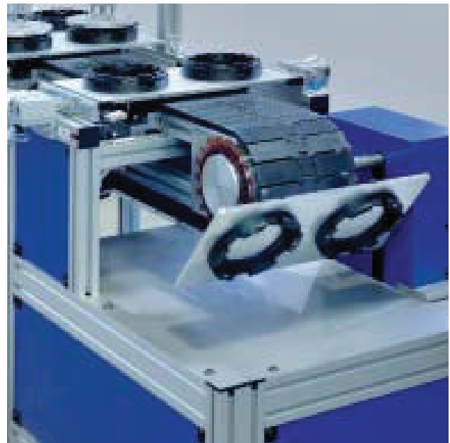
Accumulating table top chain conveyor with workpiece fixtures returning underneath
