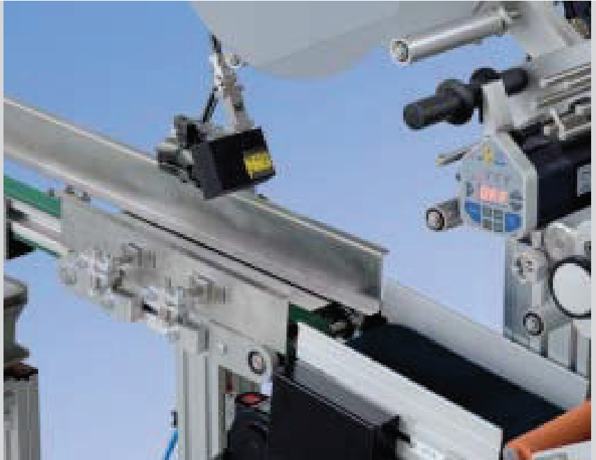
Transport and turning system with integrated CD labelling station
