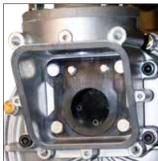
Only 4 bolts to access flap valves
